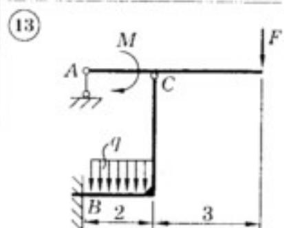
$M = 40 \text{ кН}\cdot\text{м}; q = 20 \text{ кН/м};$
