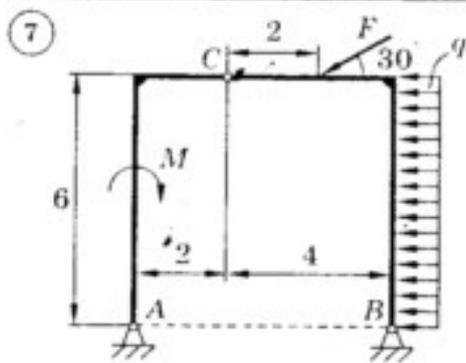
$M = 30 \text{ кН}\cdot\text{м}; q = 10 \text{ кН/м};$
