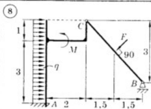
$M = 11 \text{ кН}\cdot\text{м}; q = 4 \text{ кН/м};$
