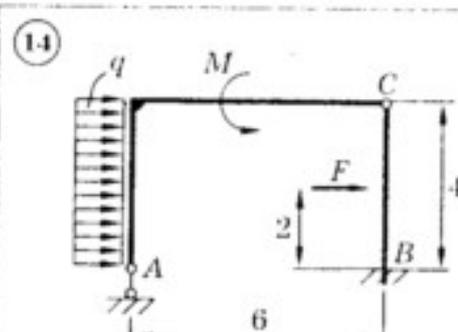
$M = 40 \text{ кН}\cdot\text{м}; q = 10 \text{ кН/м};$
