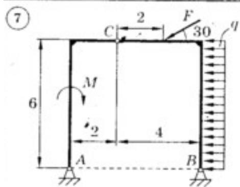
$$M = 30 \text{ kN}\cdot\text{m}; q = 10 \text{ kN/m}; F = 15 \text{ kN}$$
