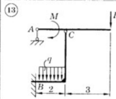
$$M = 40 \text{ kN}\cdot\text{m}; q = 20 \text{ kN/m}; F = 20 \text{ kN}$$
