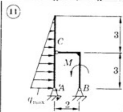
$$M = 20 \text{ kN}\cdot\text{m}; q_{\max} = 40 \text{ kN/m}$$
