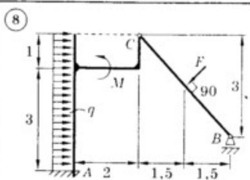
$$M = 11 \text{ kN}\cdot\text{m}; q = 4 \text{ kN/m}; F = 13 \text{ kN}$$
