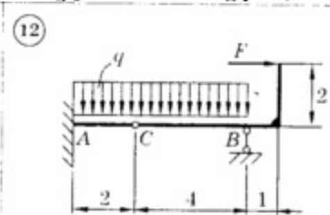
$$q = 20 \text{ kN/m}; F = 50 \text{ kN}$$
