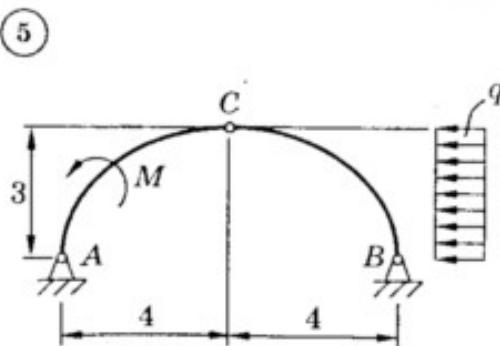
$$M = 40 \text{ кН}\cdot\text{м}; q = 20 \text{ кН/м}$$
