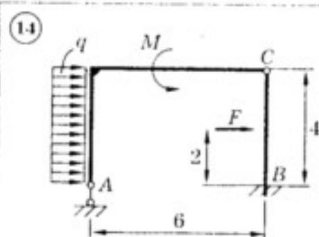
$$M = 40 \text{ kN}\cdot\text{m}; q = 10 \text{ kN/m}; F = 30 \text{ kN}$$
