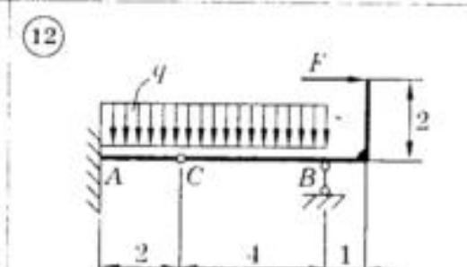
$q = 20 \text{ kH}/\text{m}$ ;  $F = 50 \text{ kN}$
