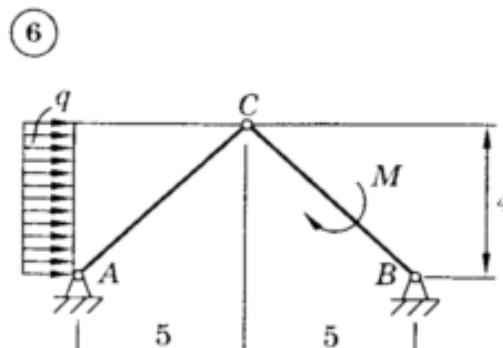
$$M = 20 \text{ кН}\cdot\text{м}; q = 30 \text{ кН/м}$$
