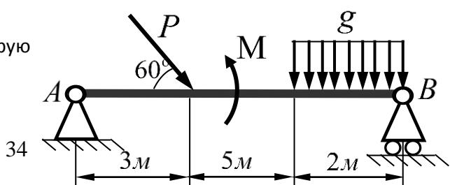
$$P = 5 \text{кН}, \quad g = 2 \frac{\text{кН}}{\text{м}}, \quad M = 10 \text{кН} \cdot \text{м}.$$
