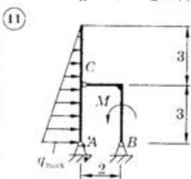
$$M = 20 \text{ kH}\cdot\text{m}; q_{\max} = 40 \text{ kH/m}$$
