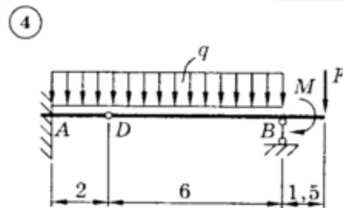
$$M = 65 \text{ кН}\cdot\text{м}; q = 20 \text{ кН/м}; F = 30 \text{ кН}$$
